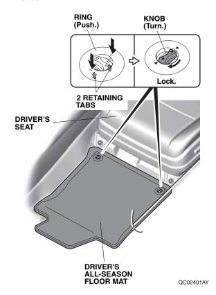
2. Install the rings in the driver's all-season floor mat over the anchors. Push the rings into the anchors to secure the retaining tabs, then turn the knobs 90° to secure the floor mat to the floor.
